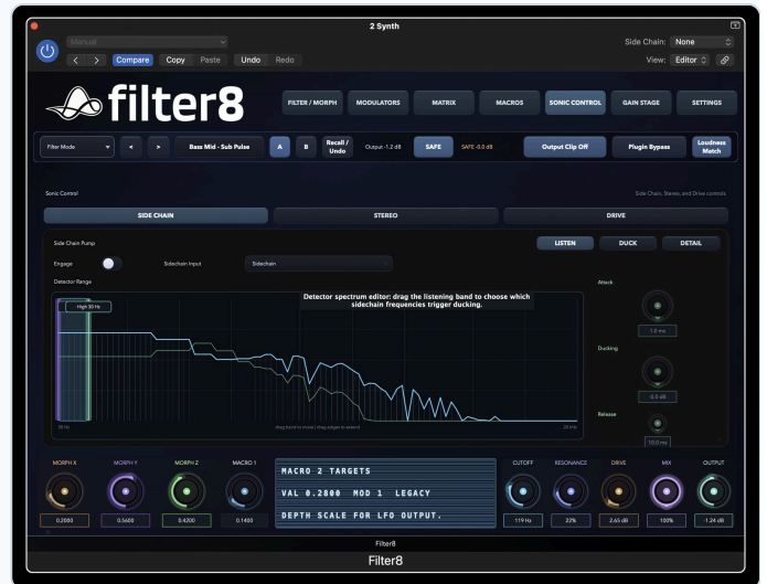
Detector spectrum: tune detector range around the energy that should control the patch.
